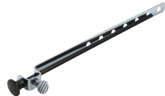
Qty: 1 set. Pop-Up lift rod and linkage kit, used for the repair and replacement of damaged or missing lavatory lift rods and clevis straps, 3/16 in. rod diameter, 11/16 in. head diameter, 8 in. rod length. RP31226CH (Chrome) RP31226SN (Satin/brushed nickel) RP31226OR (Oil rubbed bronze)
