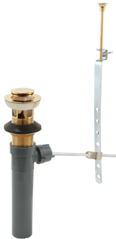
Qty: 1 set. 50/50 Construction, plastic tailpiece with metal top body and trim, features a universal fit for most sinks with an overflow, Rapid Ring pre-installed. RP31200CH (Chrome) RP31200SN (Satin/brushed nickel) RP31200OR (Oil rubbed bronze) RP31200PB (Polished brass) RP31200PN (Polished nickel)
