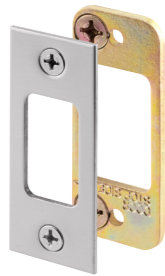
Qty: 1 set, with fasteners. 1/8 in. thick heavy gauge steel base, 2-1/8 in. hole spacing, improves security with 3 in. long screws attaching to wall stud. E 2479 (Brass finish) E 2482 (Classic bronze finish) E 2480 (Antique brass finish) E 2688 (Stainless steel) E 2483 (Satin nickel finish) E 2796 (Matte black finish)
