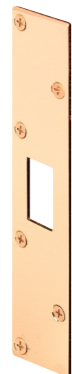
Qty: 1, with fasteners. Steel, improves security with 3 in. long screws attaching to wall stud. U 9425 (Brass finish)
